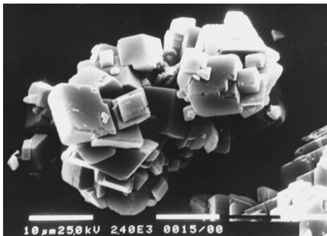
FIGURE 8 SEM image of a sample of commercial calcite powder as it came from the bottle. The faces of the crystallites appear smooth and regular.
